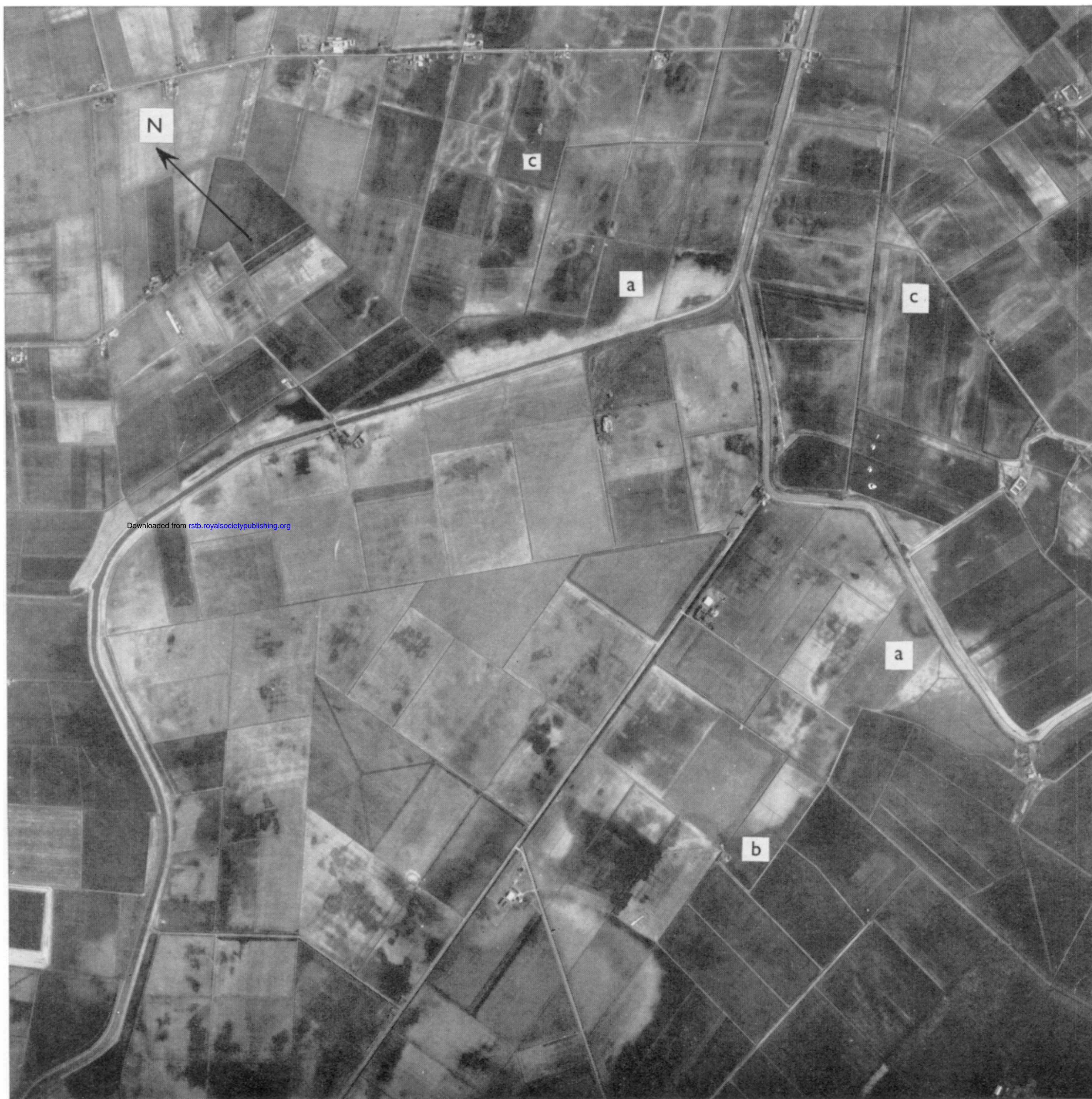
FIGURE 23. Vertical air photograph in which the northeastern part of the bed of Whittlesey Mere is shown by the white shell marl contrasting with the darker peat land round it and especially on its southern boundary with Holme Fen (b). The straightened drainage channels of the 'Old River Nene' cut directly across the meandering course (a) of the natural river (see figure 2) whose silt levées limited the northern side of the mere. At (c) there are pronounced relict creek systems apparently draining eastwards from the banks of the natural river, but their age and relationships still await investigation (cf. however Green Dyke area, Godwin & Clifford 1938). (Photograph by the Department of Aerial Photography, University of Cambridge.)
